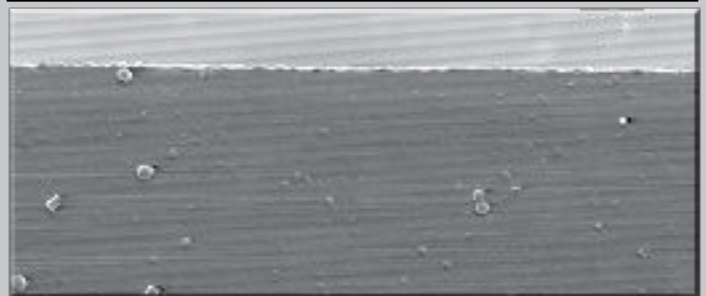
Figure 6 Si 3 N 4 Ceramic Ground with RVG WS60 Diamond
